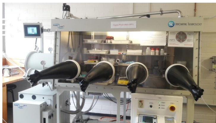
Photo 15. Glove box to make polymer solar cell and perovskite solar cell devices under desired atmosphere.
