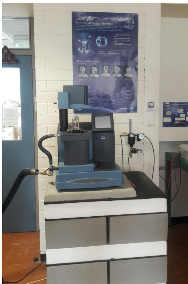
Photo 16. Dynamic Mechanical analyzer helps to understand the mechanical properties of polymers
